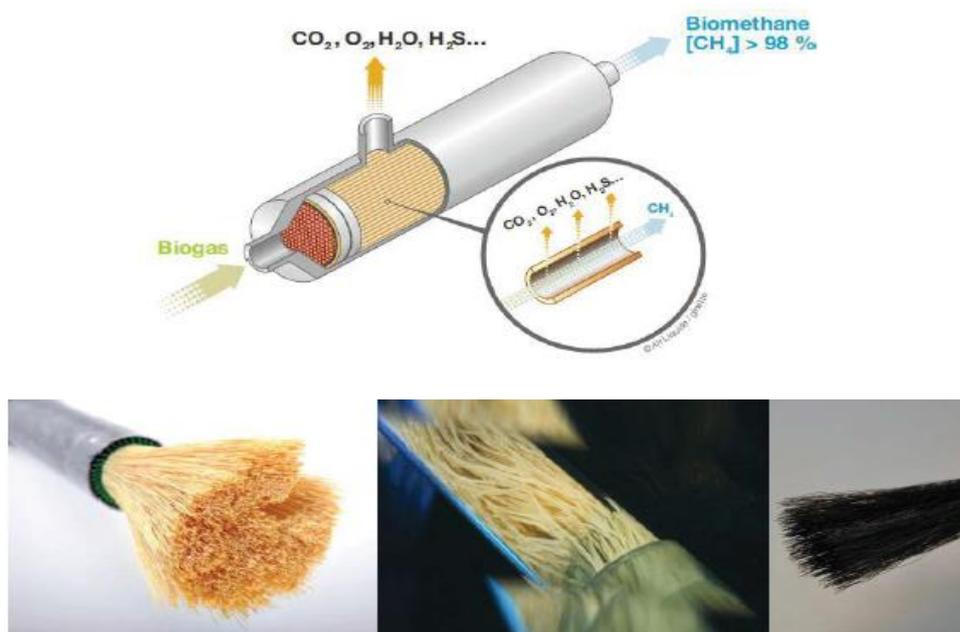
Figure 3. SCHÉMA DE L'ÉPURATION MEMBRANAIRE DU BIOGAZ
